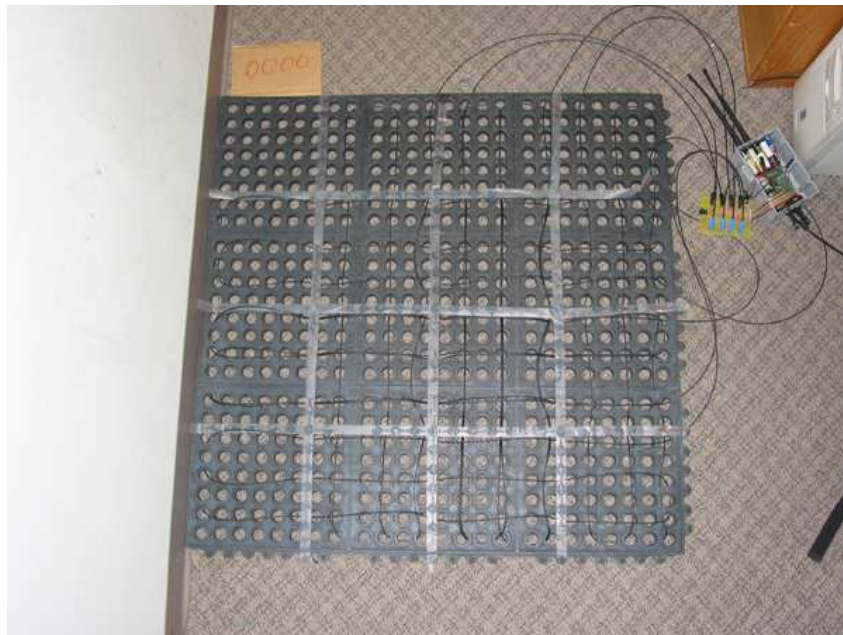
Figure 2.5: A fiber mat system with 4 \times 4 cells woven on a single mat. A complete signal channel consists of LED, fiber, darlington receiver, A/D board and wireless unit.
