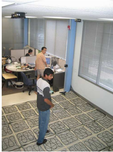
Figure 2.6: A fiber floor weaved on a hardware net.
